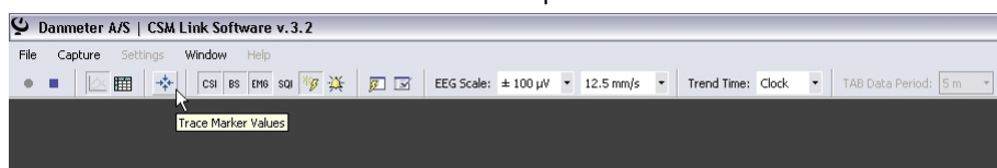
Figure 9: Use the toolbar button "Trace Marker Values" to start tracing marker values.
